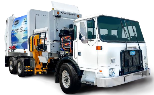
Autocar's All-Electric E-ACX with cover removed to display one of three high voltage battery packs.
